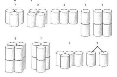
All Yuasa cylindrical cells can be connected together to form higher voltage/capacity packs. Dependent upon quantities required, almost any configuration can be achieved. Pack details are available on request.
