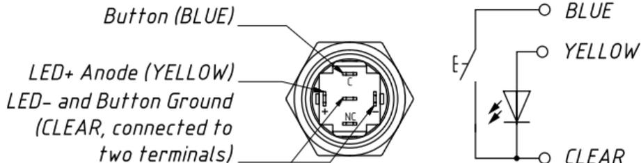
*Figure 2. Button terminals and electrical scheme*
