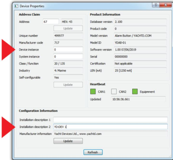
Figure 1. Programming with CAN Log Viewer
