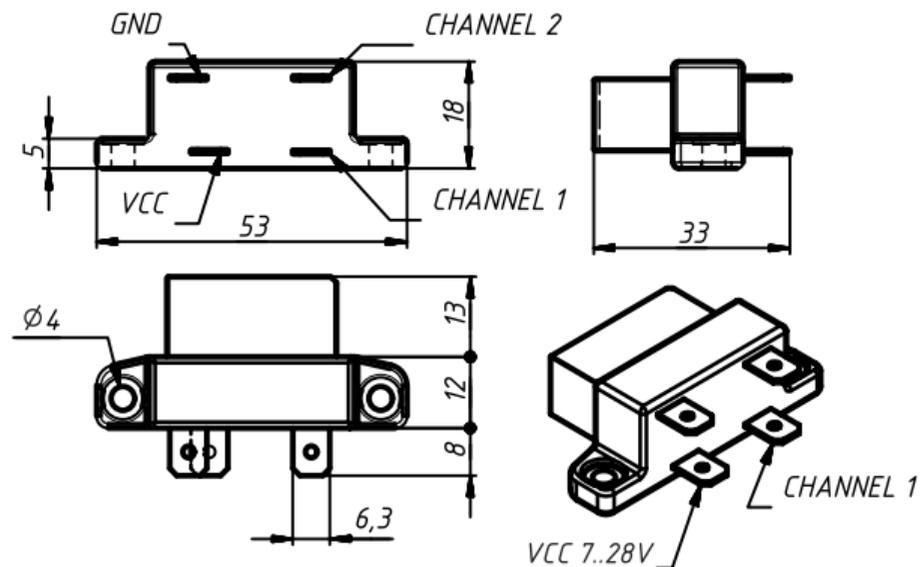
Device is equipped with four standard blade "FASTCON" terminals (6.3mm x 0.8mm). Five receptacles with insulation are supplied with the device, they are widely available in any electronics store.
