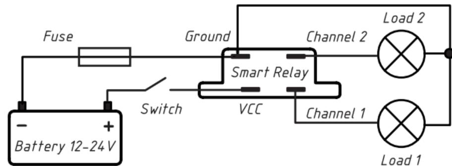
Smart switching is managed by a micro controller inside the device's case. High voltage (over 28V) on VCC terminal can cause permanent damage to the device.
