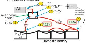
3=Output diode Voltage to domestic battery
