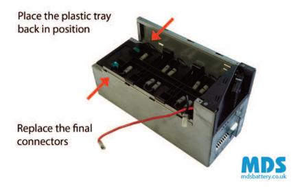
Place the last three new batteries in position
